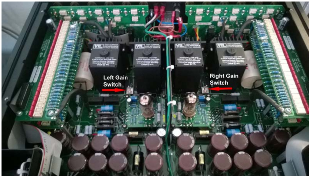
NORMAL GAIN -- switch towards back panel LOW GAIN -- switch towards front panel
